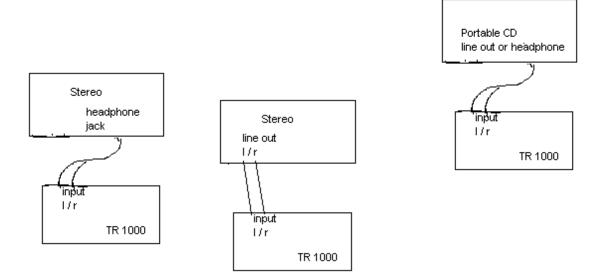
The input section requires input from one or two RCA male jacks. When connecting from a stereo source you will connect both audio jacks. When connecting from a mono source (such as an older tape recorder), you can connect to either the left or right input jack on the TR-1000.
